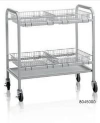
Glassware Carts. Safely transport clean and dirty labware. Come with two large or four small interchangeable vinyl-coated wire baskets and removable drip pan below the baskets to catch spills. Include 4" diameter casters (two with toe locks). Frame is welded 1" square mar-resistant, powder-coated tubular steel. Overall dimensions: 34.9" w x 19.0" d x 36.4" h. Fully assembled. Lifetime warranty. Shipping weight 43 lbs. (20 kg) △ WARNING: Cancer — P65Warnings.ca.gov (California only)
